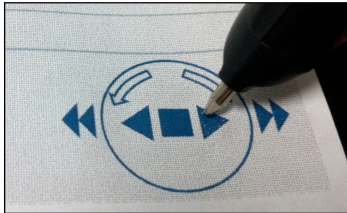
Figure 5: Video playback controls printed on Anoto pattern.
